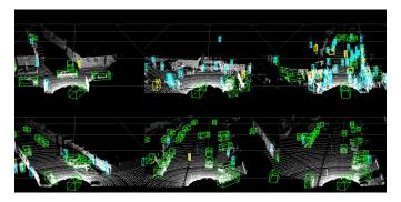
Point cloud object detection using KITTI dataset
